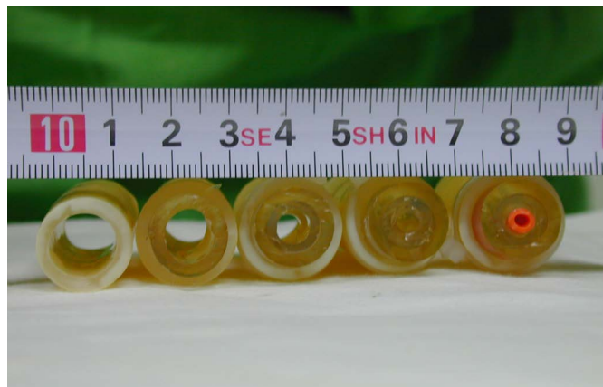
Fig. 1. Schematic (A) and picture (B) of the experiment setup and a photograph (C) of the stenosis model (grade 0 to grade 4, from left to right).
