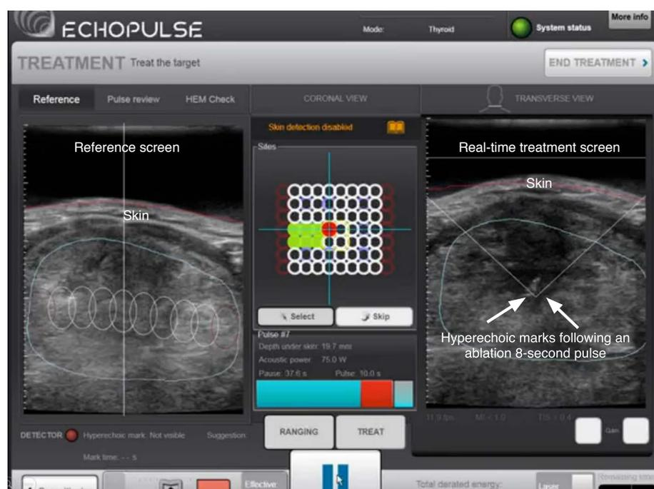
**Fig. 1.** A treatment image captured immediately after an 8-second treatment pulse. The central panel represents the bird-eye view reconstruction of the nodule. The empty circles represent the non-ablated subunits, while the filled circles represent the ablated subunits. The presence of hyperechoic marks (microbubbles) at the focal point of the high-intensity focused ultrasound beams in the treatment screen should also be noted.
